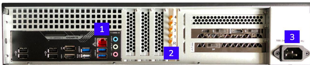
1 Network 2 SDI Inputs 3 Power
